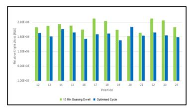
**Figure 2:** Optimised cycle shows a general increase in EI inactivation to the reduced cycle from the initial study. Only Isolator chamber locations have been compared as the Sterility Isolator was not loaded in the initial study.
