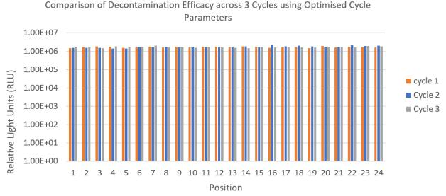
*Figure 3:* Optimised cycle shows consistent decontamination efficacy across triplicate cycles on a loaded Sterility Testing Isolator.
