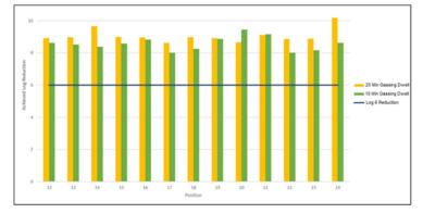
*Figure 1:* Initial investigative study results showing maintained cycle efficacy when reducing the gassing dwell phase.
